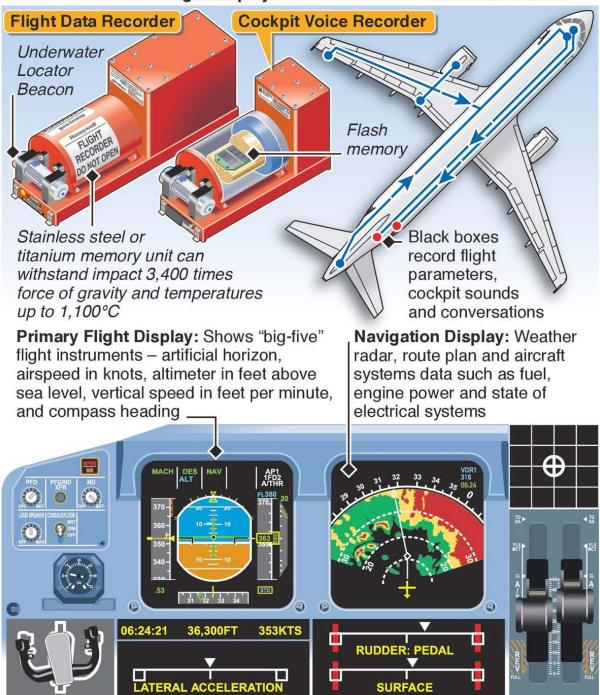
Sources: CAE Flightscape, Honeywell ED-55 Flight Data Recording System
